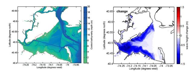
The models showed that oyster reefs significantly reduced wave height and wave energy for both storms. Wave height reduction was very sensitive to reef height, but not to reef roughness. Peak average flood level was only changed by a very small amount by the presence of reefs, and the direction of change varied by storm. Together, the sediment analysis and modeling indicate that large, well-established oyster reefs can provide protection for storms by decreasing the height and
